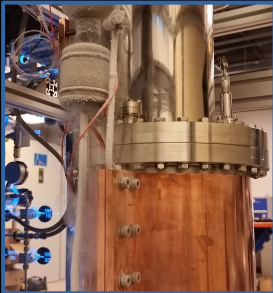
First cooling tests with the copper belt
