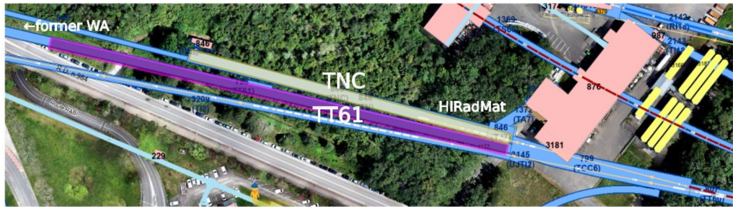
Figure 8: View of the TNC (yellow frame) and TT61 (purple frame) tunnels downstream of the extraction location in SPS LSS6. The first part of the TNC tunnel is occupied by the HiRadMat test facility, while the downstream tunnel (approximately 120 m) can be used for the beamline. The TT61 tunnel – although slightly narrower than the TNC tunnel – is currently not occupied.
