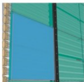
Field cage equipped with Photon Detectors (128 nm)
