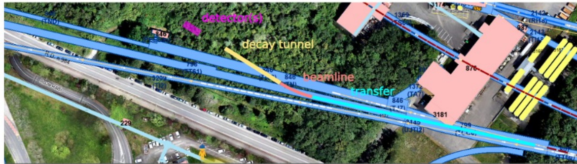
Figure 9: In the current beamline design and pending further optimization, the beamline cannot be operated successfully at a reduced bending angle. For this reason, the beamline is placed with a straight transfer and requires the excavation for the neutrino detector and the final part of the decay tunnel.
