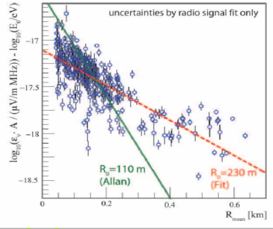
**Correlation of the radio pulse height with the mean distance of the shower axis**
