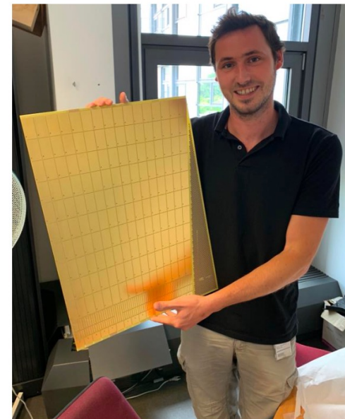
58 cm x 44 cm x 1.2 mm electrode prototype at CERN
