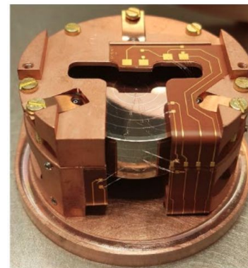
4 ionisation channels Fiducial volume ~70% Surface events rejection!
