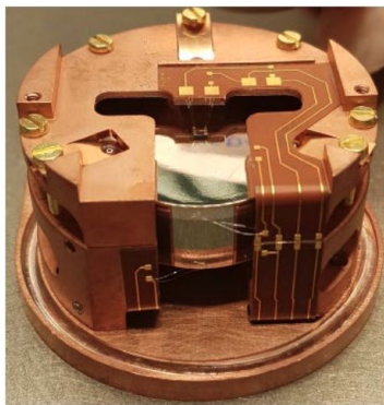
2 ionisation channels Fiducial volume ~99%
