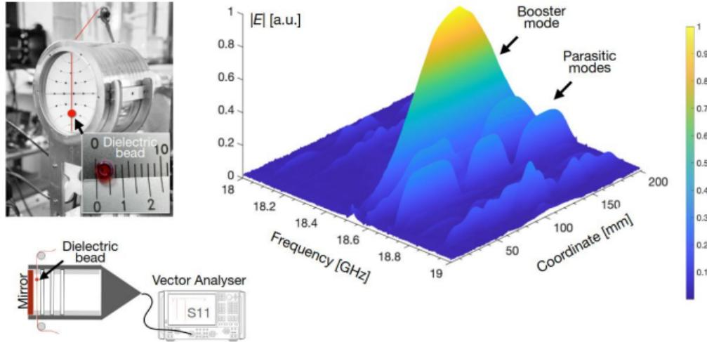
Measured E field within closed booster
