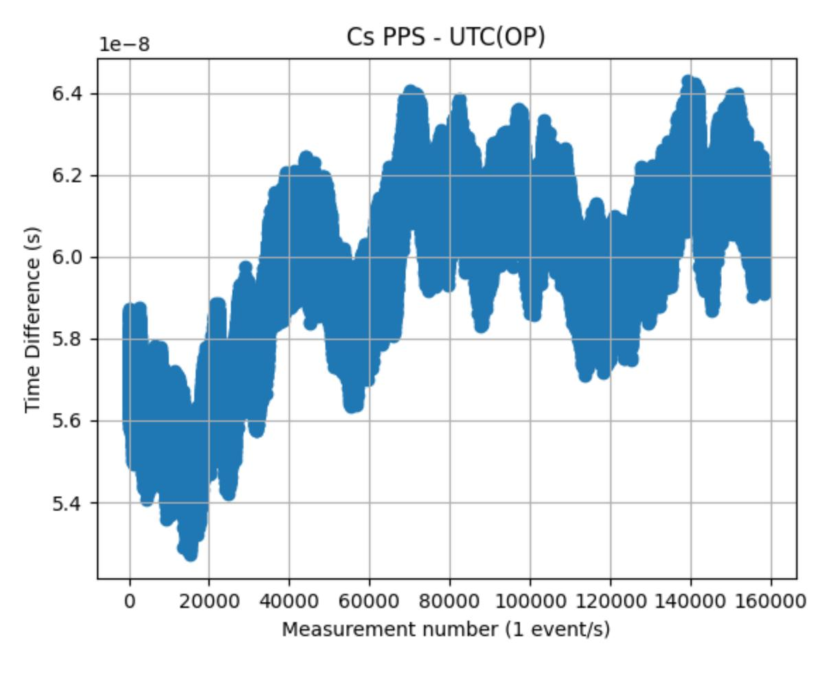
Lot of white noise (>10 times more than Rb)! Could it be due to the counter's configuration: wrong impedance? Starting another run with a 1M impedance (instead of 50k)
