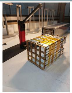
New FAZIA detection blocks have been reassembled and mounted on the electronics
