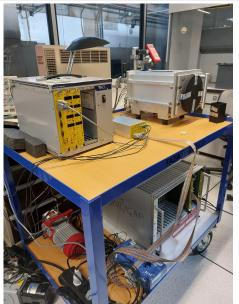
A new test bench has been realized, in order to test all detectors *before* mounting them on the FAZIA electronics.
