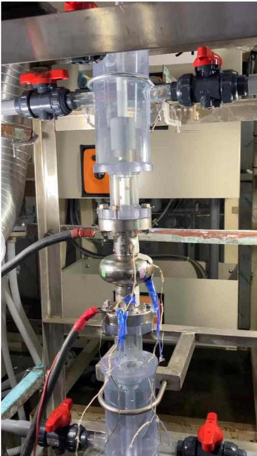
For EP process, a vertical EP setup dedicated to 3 GHz cavities was used.
