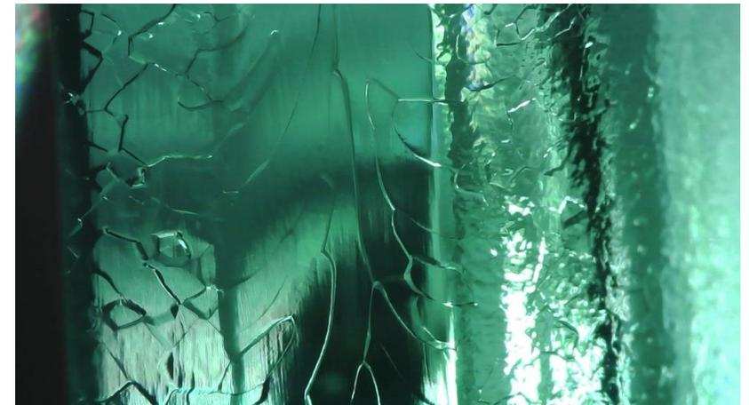
Inner surface 85 degree equator close to the heating point 90degree. No defect found.
