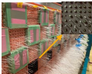
Fishing lines removal and WLS fiber insertion
