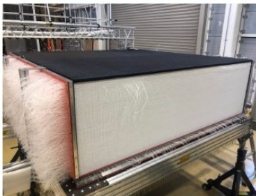
Fishing lines removal and WLS fiber insertion
