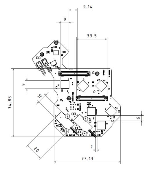
Exemple of FEB:  $6 \text{ lpGBT} \rightarrow 18 \text{ CALOROC } ??$  $S= 56 \text{ cm}^2$
