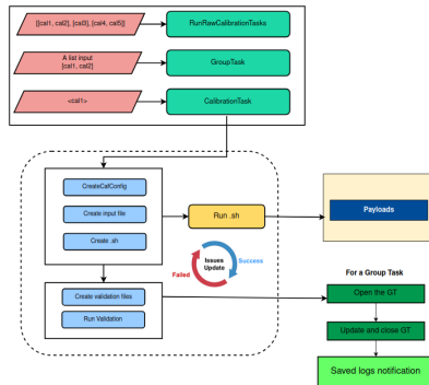
Figure 7: The execution flow of the calibration task.
