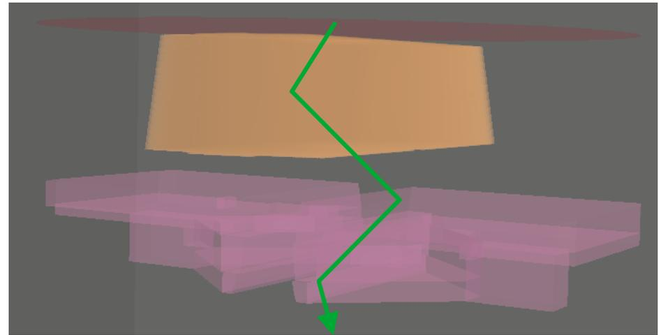
Sketch of the last vertex splitting applied to a triple Compton scattering
