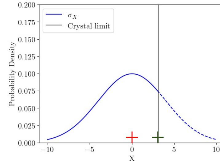
The standard deviation of the distribution is reduced and all hits that would fall out end up at the crystal's limit, closer to the original position.
