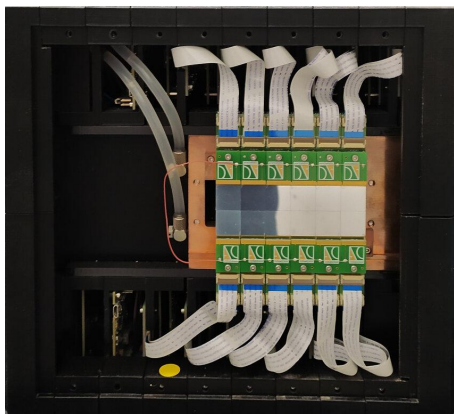
Figure 1: Picture of the TimePix detector with its cooling system.
