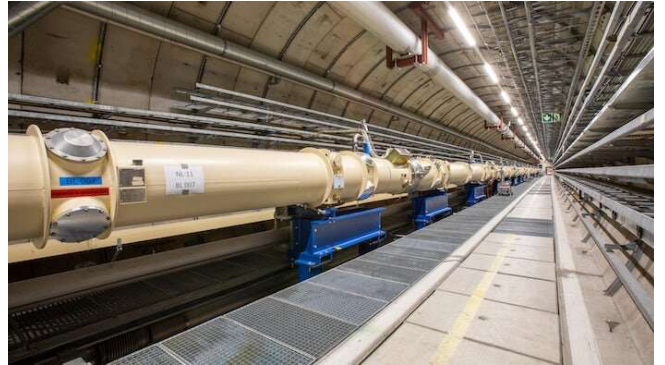
ALPSII experiment at DESY is a light shining through a wall (LSW) axion dark matter search approaching final science runs.
