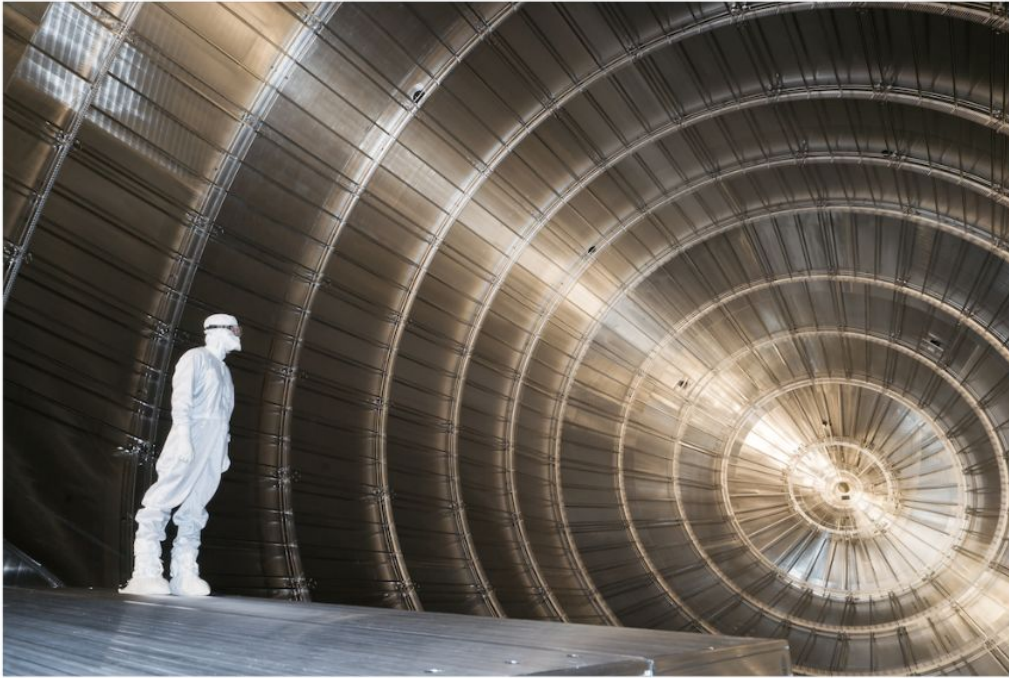
Inner electrode system Ultra high vacuum
