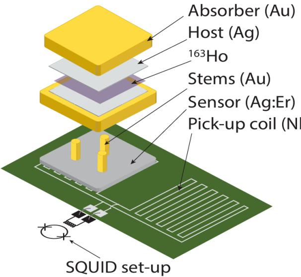
Absorber design and fabrication optimized for full energy containment
