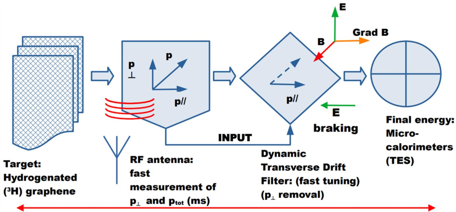
electrons near endpoint are slowed down by EM filter to an energy range of  $\sim 0\text{--}10 \text{ eV}$
