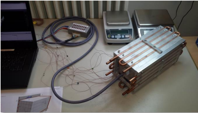
Setup of the thermal with prototype 5x5 (without cooling)
