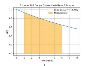
$$N_{decays} = \frac{A_{source}}{\lambda} \left( e^{-\lambda (T_{start} - t_{ref})} - e^{-\lambda (T_{end} - t_{ref})} \right) D$$
