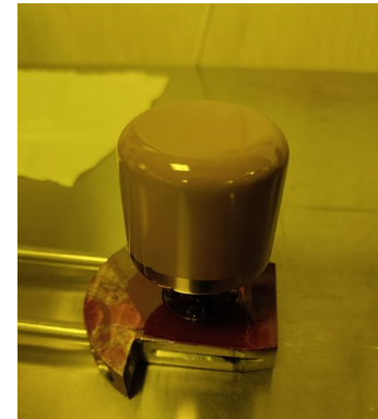
Al plated + photoresist spray coating
