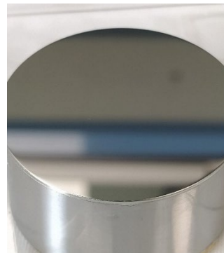
Polished surface (CMP) (Low waviness, low roughness)
