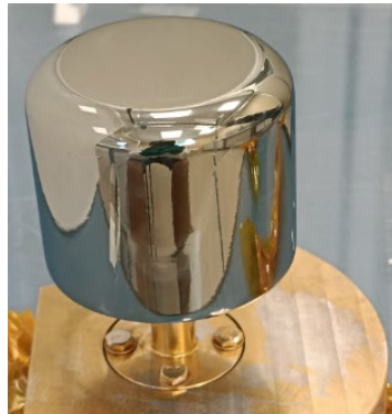
50mm d, 50mm h, n-type crystal, AlGe PLM junction, Li core
