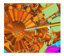
Telescopic movement of the beamline to change detectorstarget distance working in high-efficiency configuration: continuous range from 0 (nominal) to - 55 mm (high eff.)
