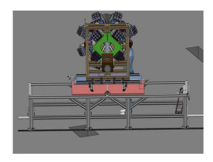
The majority of the elements of the supporting structure are made in aluminium or are aluminium profiles (AP)
