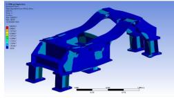
Deformation analysis performed assuming a weight of 10 tons (10<sup>5</sup> N) Deformations are not uniform on the surface:
