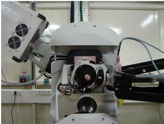
Detector installed on the diffractometer
