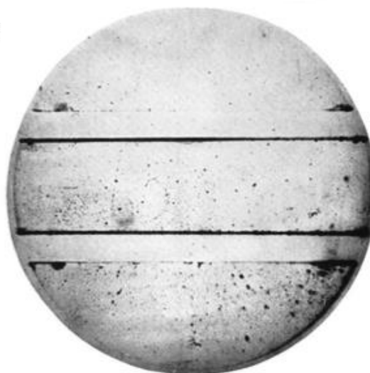
FIG. 1. A 63 million volt positron ( H_p = 2.1 \times 10^6 gauss-cm) passing through a 6 mm lead plate and emerging as a 23 million volt positron ( H_p = 7.5 \times 10^6 gauss-cm). The length of this latter path is at least ten times greater than the possible length of a proton path of this curvature.
