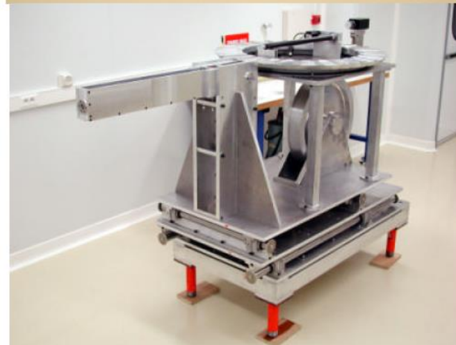
"Carousel" brick dispensing and storage system
