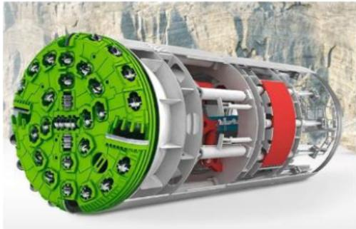
Tunnel Boring Machine (TBM)
