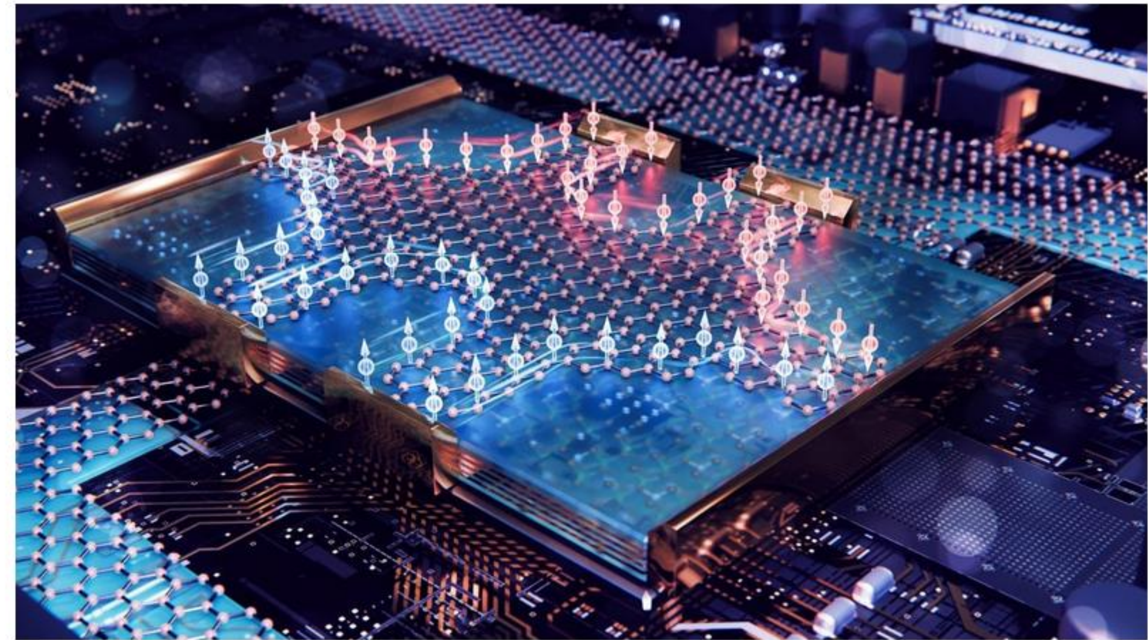
Artist's impression of the quantum spin Hall effect in a graphene-based spintronic device, integrated in a chip. The blue and red spheres are spin-up and spin-down electrons traveling along the edge of the graphene. Underneath the graphene lies the layered magnetic material CrPS4. Credit: ScienceBrush, Talieh
