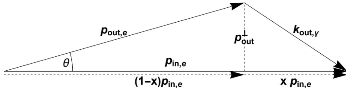
$$\begin{aligned}\Gamma_{\text{VC}} &\equiv \int dx \frac{d\Gamma_{\text{VC}}}{dx} \\ &= \frac{\alpha}{2p} \int \frac{dx dp_{\text{out},\perp}^2}{px(1-x)} \delta \left[ \omega_{\text{LIV}}^{\text{VC}}(x) - \frac{p_{\text{out},\perp}^2}{2px(1-x)} \right] \overline{|\mathcal{M}_{\text{LIV}}^{\text{VC}}|^2}\end{aligned}$$
