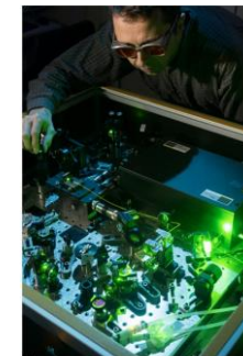
The LNE's femtosecond laser, used for practical realization of the meter
