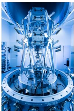
The LNE's Kibble balance, used to produce the value of the Planck constant, h
