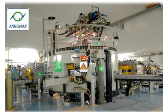
Figure 8: ARRONAX cyclotron C70XP
