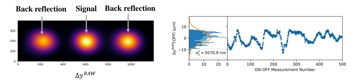
• By making « OFF-OFF » measurements (without laser pump pulse), we measure the spatial resolution of  $\Delta y^{RAW}$ .
