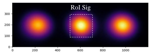
The measured displacement  $\Delta y_{\text{mes}}$  depends on the size of the RoI
