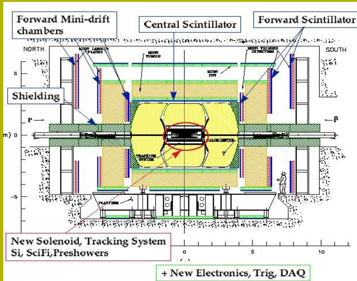
The D0 experiment is focused on precise studies of interactions of protons and antiprotons at the high energies. It is comprised of three major parts: the tracking system, the calorimeter, and the muon system.
