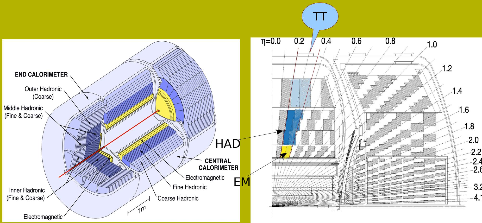
The liquid argon calorimeter consists of 3 units: the Center Calorimeter (CC), and the two End-cap Calorimeters (EC).
