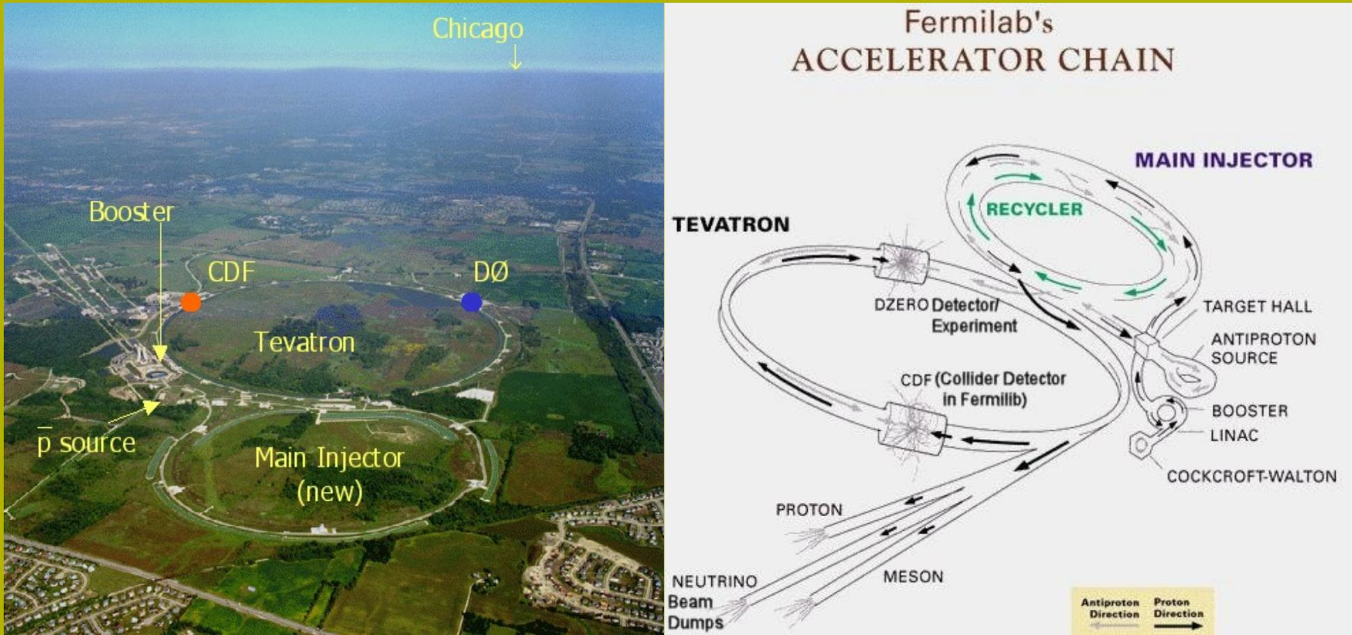
The Tevatron accelerates protons and antiprotons in a 6.3 km ring to energies of up to 1 TeV each.
