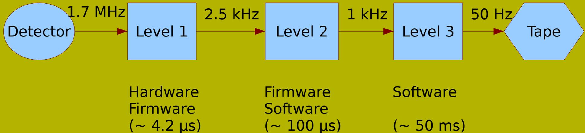
The D0 trigger system consists of 3 levels:
