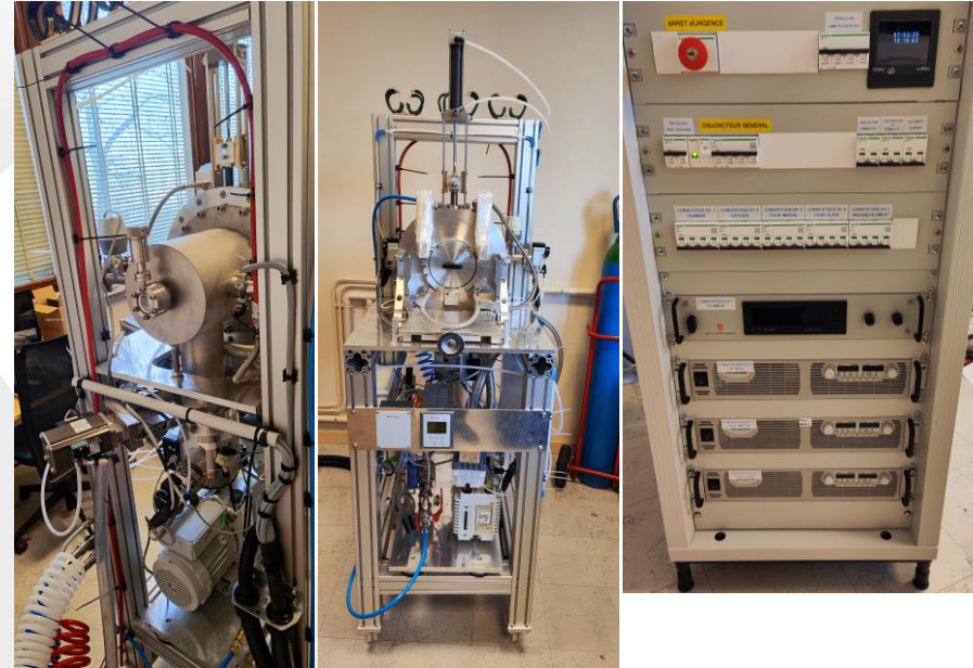
Thermal test bench: thermal measurements (16 sensors + pyrometer) and filament developments.
