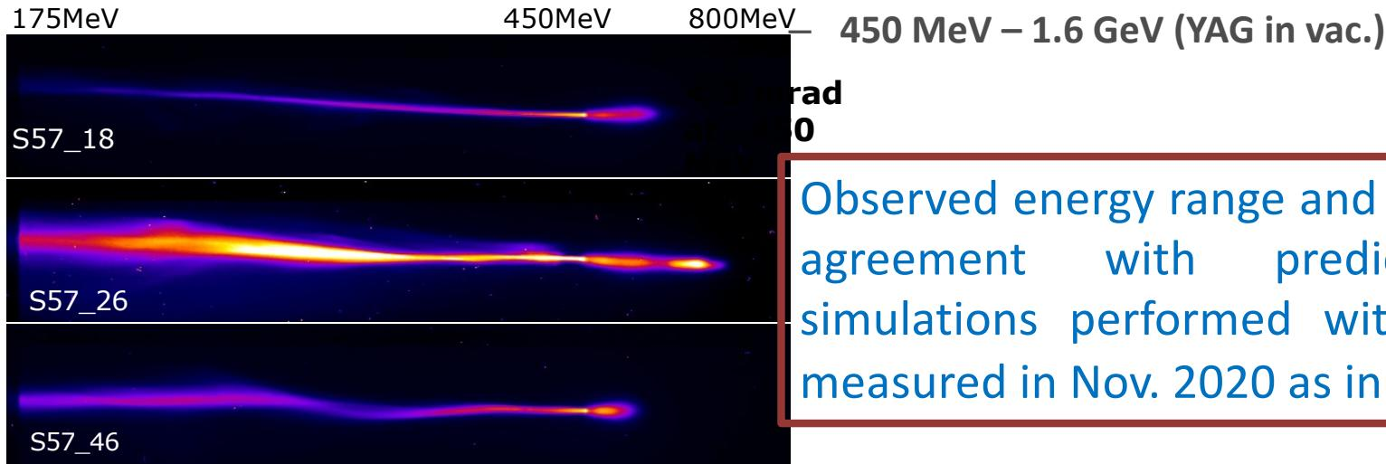
Observed energy range and distribution in agreement with predictions, from simulations performed with focal spot measured in Nov. 2020 as input
