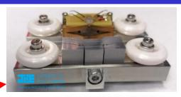
2021: Successful test of 1 piezo motor at 5 K and 5.3 T (ALP magnet in DESY)
