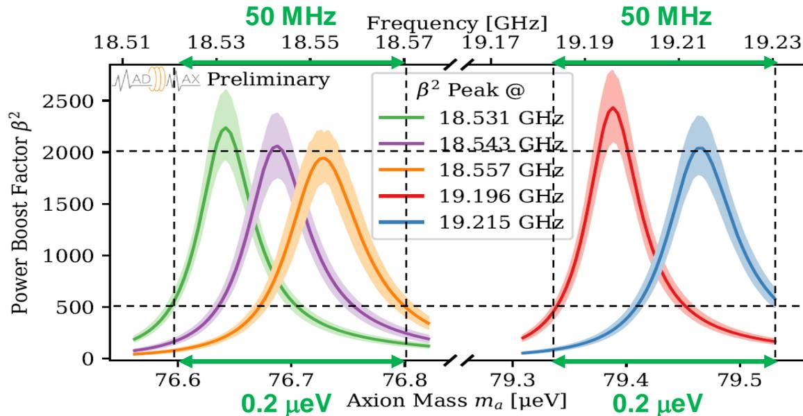
**Demonstrating the scanning capacity of MADMAX booster**
