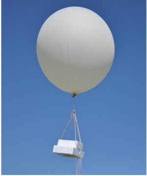
radio sounding by a balloon launched from Tenerife
