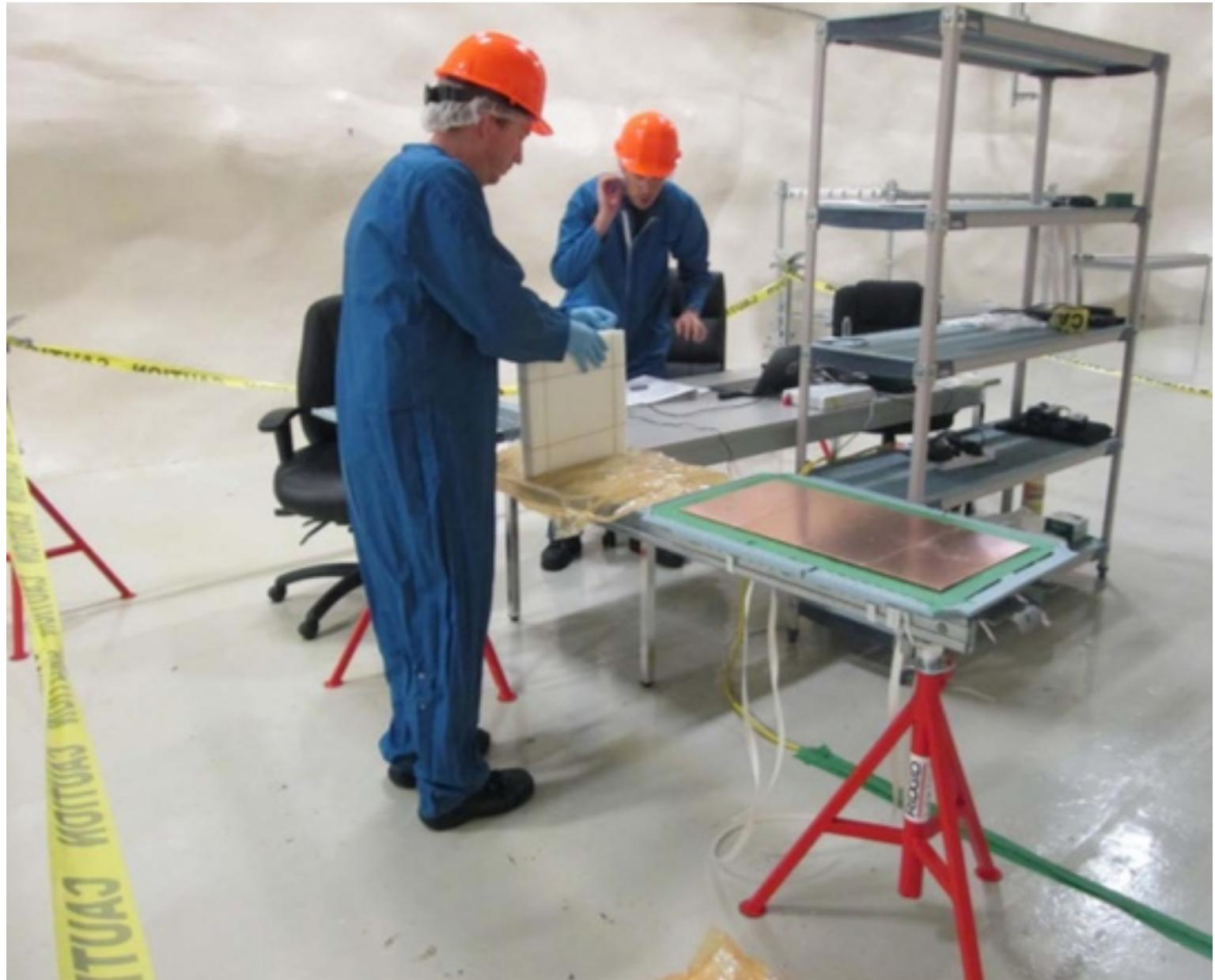
Exposed 8 HDPE and 2 Cu samples in 4 locations underground
