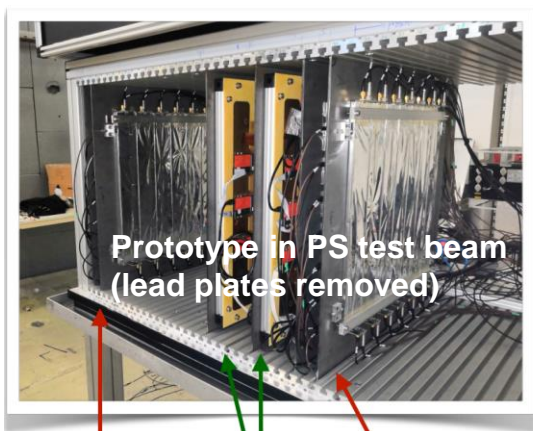
2 scintillator layers (x & y) 2 Micro-Megas 2 scintillator layers (x & y)
