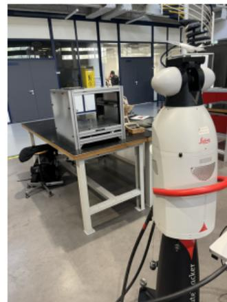
Checking the test bench geometry with a laser
