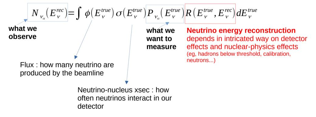
$$N_{v_{\alpha}}(E_{v}^{rec}) = \int \phi(E_{v}^{true}) \sigma(E_{v}^{true}) P_{v_{\alpha}}(E_{v}^{true}) R(E_{v}^{true}, E_{v}^{rec}) dE_{v}^{true}$$
