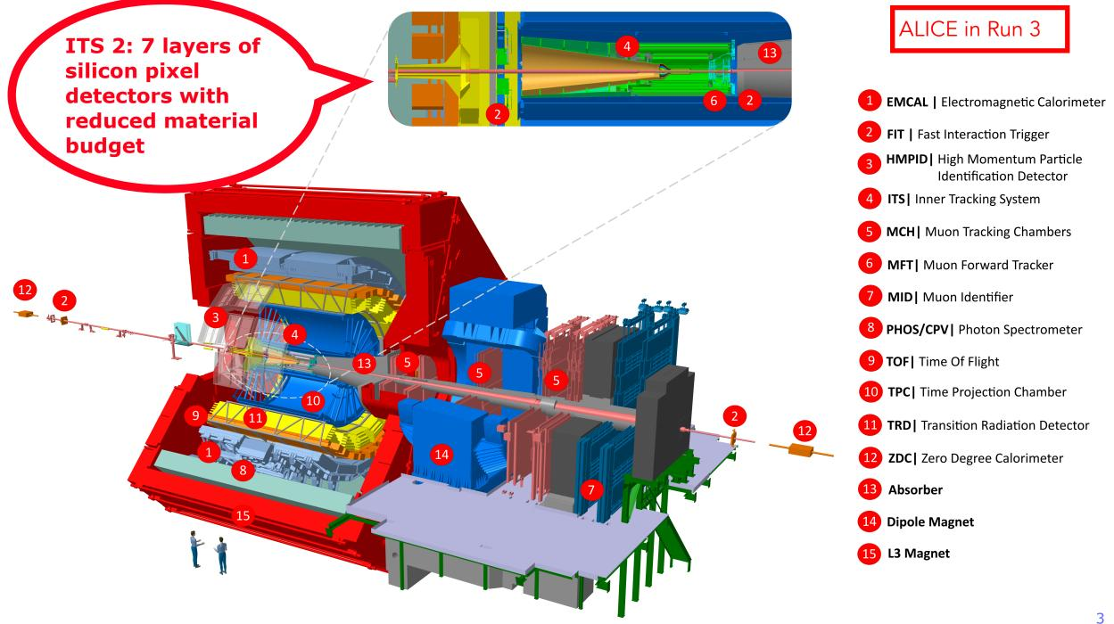
ITS 2: 7 layers of silicon pixel detectors with reduced material budget
