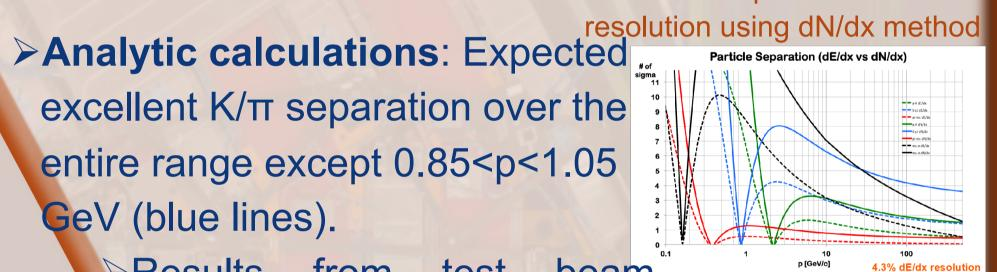
Results from test beam analysis proved that using the dN/dx method gives a resolution 2 times better .... than the dE/dx method in " agreement with the analytical
