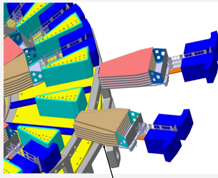
3D drawing of the insertion of two adjacent stacks of six ME0 modules (pink/brown) into the muon system.
