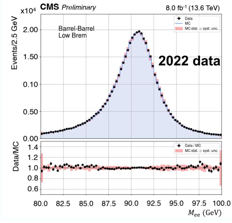
ECAL energy measurement: shifted in DATA to match the SIM peak position **smeared in SIM** to match DATA resolution
