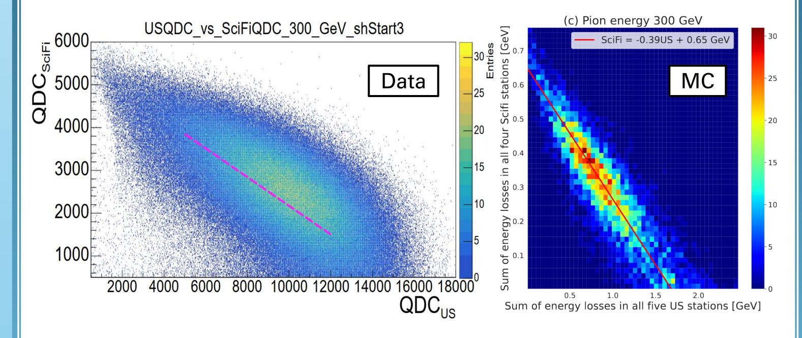
Showers starting late in the target (SciFi4) tend to cause signal saturation in the first US station and need ad-hoc calibration constants.
