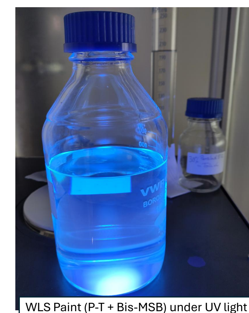
WLS Paint (P-T + Bis-MSB) under UV light
