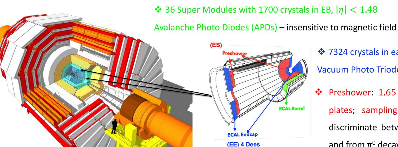
• 36 Super Modules with 1700 crystals in EB,  $|\eta| < 1.48$
