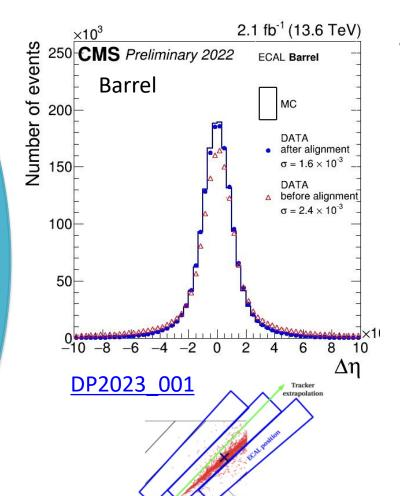
Performed using low bremsstrahlung electrons from Z boson decays
