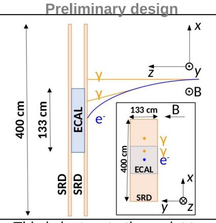
This is just a starting point to study the detection process, without considering a specific geometry of a future instrument
