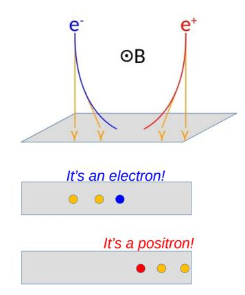
Since cosmic-ray experiments typically operate in Low Earth Orbits (LEO), we can exploit the particle bending due to the **geomagnetic field**
