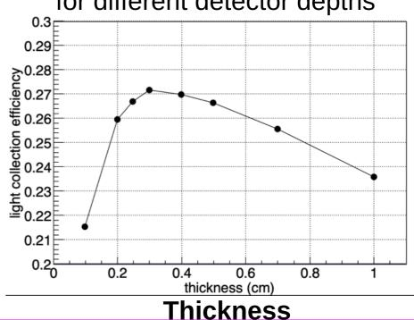
A depth of 3 mm maximizes photon collection efficiency against selfabsorption in the crystal and optical photon losses at crystal edges
