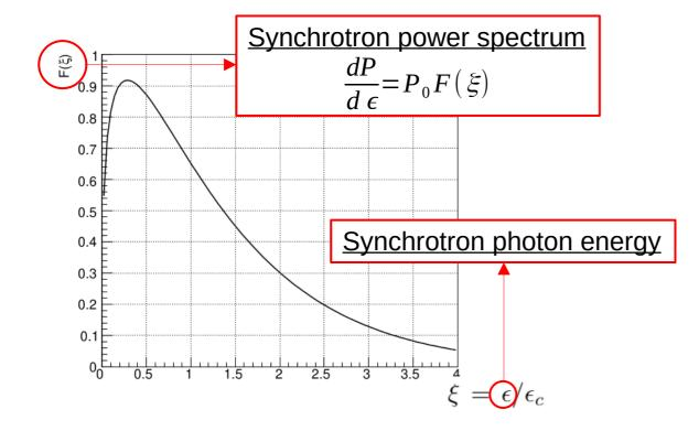
Average number of y reaching the detector  $\langle N \rangle = \langle \frac{dN}{dl} \rangle L = \frac{5\sqrt{3}}{6} \alpha \gamma \sqrt{\frac{2\Delta x}{R}} = 4.51$ Critical energy of synchrotron emission  $\epsilon_c = \frac{3}{2} \hbar c \frac{\gamma^3}{R} = \frac{3}{2} \frac{\hbar eB}{m^3 c^4} E^2 = 26.78 \ keV$
