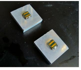
Different <u>roughness of crystal surface</u> will be tested in laboratory and with simulations to maximize light collection efficiency
