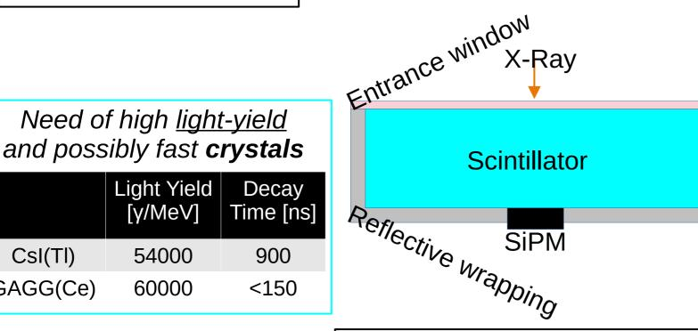
Need of a large-area and high photodetection efficiency SiPM Need of high <u>reflectivity</u> and low <u>X-absorption</u> coating
