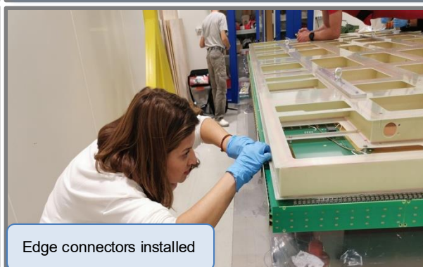
Attach the composite frame to the CRU assembly
