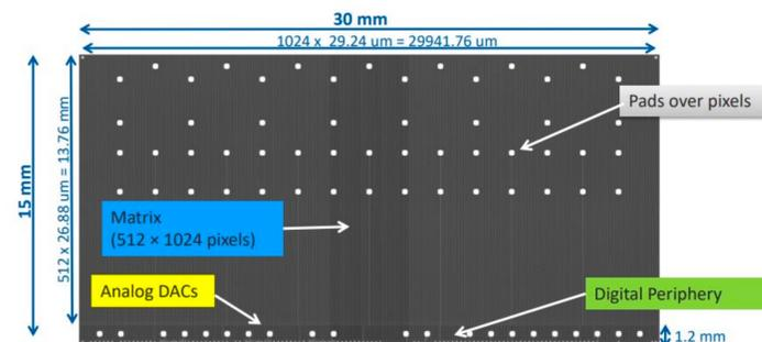
ALPIDE is the pixel sensor used. It is using 180 nm technology, containing 1024 x 512 pixels in a single sensor.
