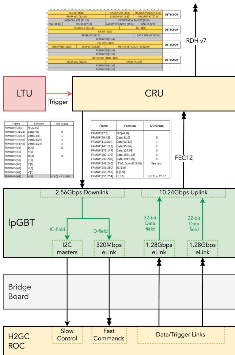
In ALICE FoCal, the data flow from/to H2GCROCs is done via data concentration ASICs (IpGBT, ECON-D, ECON-T)
