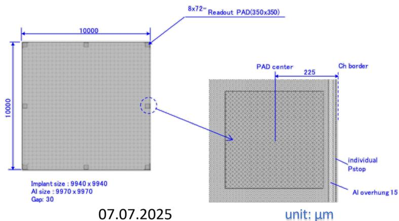
One selected pad sensor is made by Hamamatsu. The main sensor module is 9 cm x 8 cm, with 72 main cells and 2 calibration cells.
