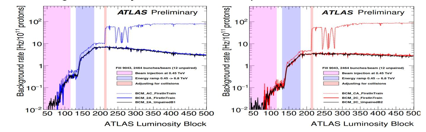
The new algorithms 2A' and '2C' with two early hits enable a beam background measurement on some paired bunches of colliding trains grouped in the 'First In Train' bunch group.
